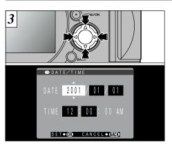
Use the "◀▶" button to select the desired item and then use the "▲" and "▼" buttons to correct the setting.
